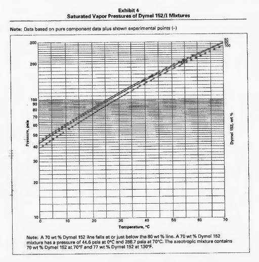
Exhibit 5 Saturated Vapor Pressures of Dymel 152/I Mixtures—Experimental Data
