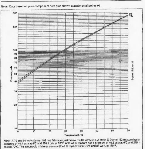
Exhibit 4 Saturated Vapor Pressures of Dymel 152/B Mixtures
