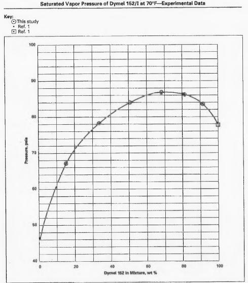
Exhibit 1 Saturated Vapor Pressure of Dymel 152/I at 70°F—Experimental Data
