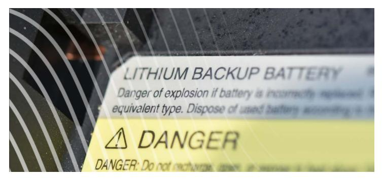
Lithium batteries can overheat and catch fire under certain conditions and the fires can be hard to extinguish and may produce toxic fumes. As a result, there are a number of requirements associated with shipping lithium batteries.
